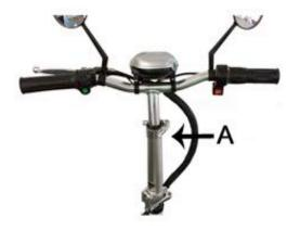
Standing behind the EMU Trike™, open the upper quick-release lever "A" to loosen it so that you can adjust the handlebars to the left and right so that they are straight. Once the handlebar is straight, you want to tighten and secure that same quick-release lever "A" to lock the steering into place.
