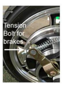
NOTE: Make sure that when the brakes are engaged, the wheel is not able to turn.
