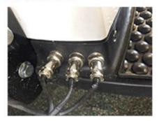
Be sure to match the pins of the plugs to the holes of the sockets by aligning the notches.
