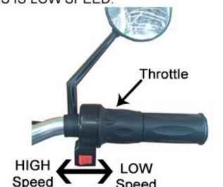
The throttle is a twist grip. To increase speed up to 8mph in the LOW speed, SLOWLY twist the throttle down toward you.
