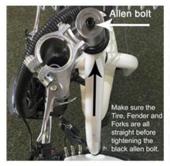
Stand behind the EMU Trike™ and adjust the tire, fender and forks until you can visually ensure that all are aligned perfectly straight. Once you are sure they are straight, use the large allen key/wrench to tighten the black allen bolt securely.
