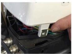
NOTE: Be careful not to let these tension clips fall into the battery area when lifting the Battery Cover. If this happens, you can use a magnetic wand to retrieve them easily. (Magnetic Wand not included in the tool kit.) To put a fallen clip back on, using your thumb and forefinger, squeeze the clip so that it is as tight as possible. (You will notice that one side of the tension clip has a wider hole than the other side.) Slide back onto the tab with the wider hole facing the outside.
