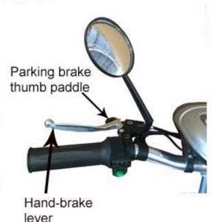
NOTE: When parking brake is set, the throttle will NOT provide power. (This is a safety feature.)
